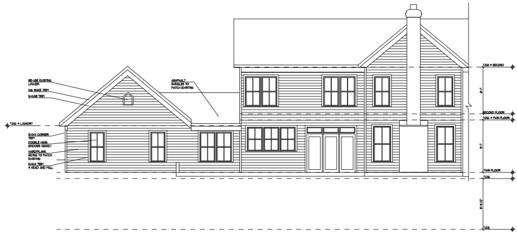
PROPOSED PARTIAL REAR ELEVATION 1/4" = 1'0"
